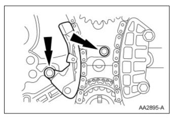
11. Remove the primary chain and sprockets as an assembly.
