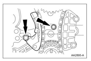
10. Using the Crankshaft Holding Tool, prevent the crankshaft from turning, tighten the jackshaft sprocket bolt
