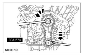
10. Remove the 2 bolts and the primary chain tensioner.
