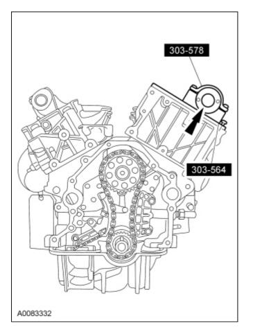
9. Using the Crankshaft Holding Tool, prevent the crankshaft from turning, remove the jackshaft sprocket bolt.
